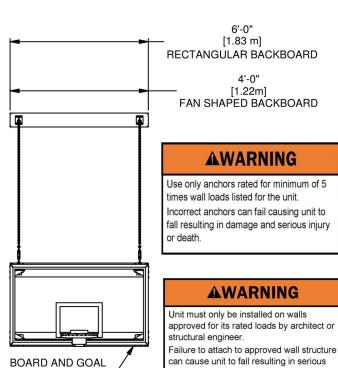
NOTE: FOR UNITS OVER 12' [3.66m] F.O.B., REFER TO INSTALLATION INSTRUCTIONS SUPPLIED WITH THE PRODUCT. IF INSTRUCTIONS ARE NOT AVAILABLE, CONTACT THE MANUFACTURER FOR CORRECT DIMENSIONS.
