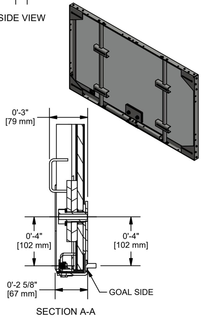
MATERIAL IS 1/2" THICK TEMPERED GLASS WITH STEEL FRAME AND STEEL STRUT MOUNT BRACKETS.
